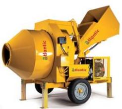
Atlantic Hydraulic Concreter Mixer is a self-loading mixer with hydraulic bucket to ease loading on construction sites. It comes with 23 HP Lombardini diesel engine which enable homogeneous mixing of cement and aggregate to produce concrete suitable for foundations and floor slabs works.
